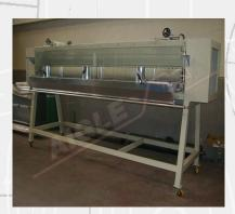
A doctor blade opposed to the cylinder is used to adjust powder output. A rotating brush is mounted opposed to the cylinder and is used to remove powder and distribute it on the fabric underneath it. Brush speed is variable and controlled by the inverter. The unit can be inspected through Plexiglas panels.
