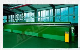
The Infrared / Hot Air Oven mod. FIR/AC12 is divided into four bays of three meters each and is heated with a combination of infrared and hot air. Each bay is equipped with stainless steel finned pipe electric batteries, air distribution ducts and recirculating fans. The infrared system consists of radiant lamps mounted on the oven's upper panel.
