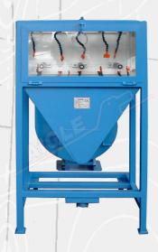
The Suction & Pre-Cleaning Group mod. PRCP and mod. Jet-Matic is placed after the flocking machine to ensure a good pre-cleaning of the profile prior to its entrance in the oven and also to avoid excessive dispersion of flock during the various working phases.
