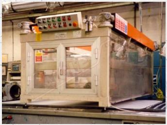
The Flocking Unit for Rotary Printing mod. TC2/COMPL is placed on the shoulders of a rotary screen printing machine. At the point where fabric and conveyor belt split, a suction blade for preliminary cleaning is located; final cleaning is performed by the brushing machine located at the oven outlet.
