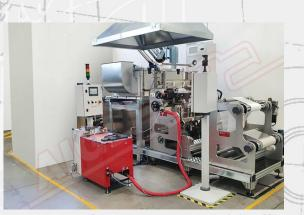
Coagulation lines are used for the production of filters and synthetic leather. This is a wet process. The substrate is first impregnated or squeegeed or slotted and then placed in contact with water diluted with other chemical compounds.
