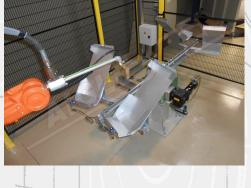
With this cabinet, it is possible to flame a variety of objects of different shapes. The process is completely automatic and it is done by robot. The objects are fixed in place on a rotating table: the operator places the object, then the table rotates to the flaming position; the other side is ready for the loading/ unloading operations and the opposite side is ready for the automatic flaming process.
