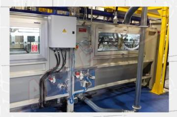
AIGLE has developed several flocking plants for Cast Iron Bell Insulators over the years. The insulator is flocked at the opening to avoid friction with other material that is then expected to contact it during use. The flock is then applied precisely and uniformly.
