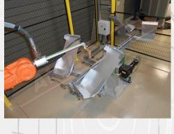
The booth can handle a wide variety of objects of different shapes. The process is fully automatic and is carried out by means of a robot. The workpieces to be treated are placed on a rotating table: the operator places the object there and the table rotates, bringing it to the automatic plasma treatment position; in the other position, the workpiece is ready for the loading/unloading operation.
