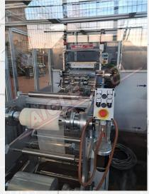
The Combination Bench mod. BSR/SLOT is designed to be able to use various coating techniques.
