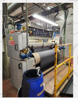
This line's **direct coating process** can be made **with one or two heads coated fabric**.
