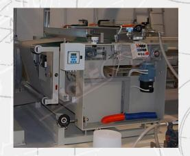
The Coating Head mod. BSR-T has been designed and built so that different coating techniques can be employed.
