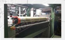
The **Rotary Screen Coater mod. B\$1** is used to coat and print fabric (with pigments, resin and adhesives) and for pattern flocking.
