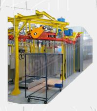
Over the years, **AIGLE** has developed several Flocking Equipment for Metallic Springs, used mainly in the automotive industry. The flocked springs are used in the systems for opening doors. The flock reduces the noise in the passenger compartment and helps the sliding of the spring inside its seat.
