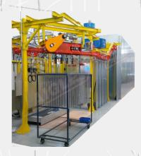
Over the years, **AIGLE** has developed several painting equipment for metallic springs, used mainly in the automotive industry. The painted springs are used in the systems for opening doors. The paint protects the spring from wear and tear over the time.
