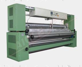
The Coating Machine mod. BSR/C is used to coat on paper (with resin and/or adhesives).
