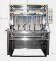
A very precise peristaltic pump applies glue to the brushes. The cabin is equipped with rear inspection doors for easy cleaning, maintenance and filter replacements. An internal light is also provided.
