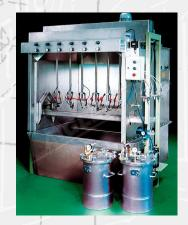
The Adhesive Application Cabin mod. ADP6 is completely built in stainless steel and is equipped with anti-spark exhausters for adhesive fumes.
