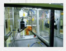
The cabinet is equipped with an electro-pneumatic flocking system mod. ESP (see the relative brochure) and with an automatic sieving and flock recovery system.
