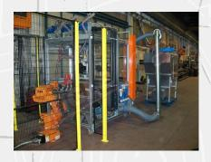
With this cabinet, it is possible to flock a variety of objects of different shapes. The process is completely automatic. The flocking gun is placed on the arm of a robot so that specific movements can be registered and easily reproduced. The objects are supported by a translating table: the operator places the object, then the table translates to the flocking position.
