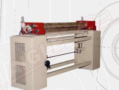
The Blowing/ Embossing Machine mod. AP1 is used to emboss flocked fabric. It must be placed between the flocking unit and the oven in order that it operates while the adhesive is still wet. The embossing effect is obtained by blowing air through rotary screen holes.
