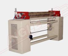
The Blowing/Embossing Machine mod. AP1 is used to emboss flocked fabric. It must be placed between the flocking unit and the oven in order that it operates while the adhesive is still wet. The embossing effect is obtained by blowing air through rotary screen holes.
