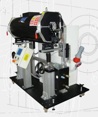
The Pre-Vulcanization Unit - mod NIRV 101 has 6 sections. Each section has two infrared lights where each lamp has an length 960 approx. of mm. The temperature of each be zone can adjusted separately via the PLC system.
