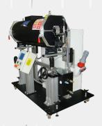
The Pre-Vulcanization Unit - mod NIRV - 101 has 6 sections. Each section has two infrared lights where each lamp has an approx. length of 960 mm. The temperature of each zone can be adjusted separately via the PLC system.
