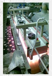
**Infrared Pre-Drying Oven** has been designed for different purposes:
