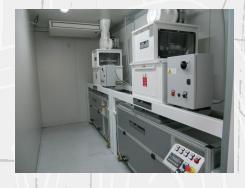
The containing/ dosing group is a special flock container on wheels. A brush equipped with a speed control is mounted at its base. Flock feeding from the brush to the flock/ air mixer is constant and adjustable.
