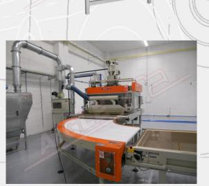
The **Flocking Machine mod. TT2** is designed to flock objects and flat surfaces.
