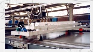
The Flocking Trolley mod. TCR/COMPL has to be assembled on the end shoulders of a flat screen printing machine.
