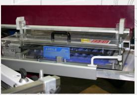
Two or more **Flocking Machines mod. TO/S** can be fitted on a carousel printer and used for multicolor flocking.
