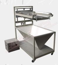
The **Flocking Machine mod. TO** is designed to flock t-shirts and can be mounted on common carousel printers. It can be supplied in two different versions, with or without flock collector or suction unit.
