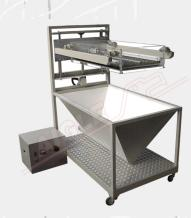
The **Flocking Machine mod**. **TO** is designed to flock t-shirts and can be mounted on common carousel printers. It can be supplied in two different versions, with or without flock collector or suction unit.
