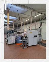
The coating system for fabric pre-treatment for digital printing, consists of doctor-blade coating on a fabric to increase the printing quality digitally done.
