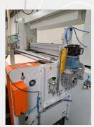
The coating system for fabric pre-treatment for digital printing, consists of doctor-blade coating on a fabric to increase the printing quality digitally done.
