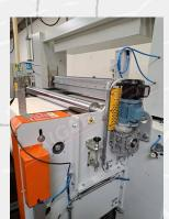
The system is equipped with an advanced tension control system in order to compensate for the continuous coating feed even in case of discontinuous belt feed.
