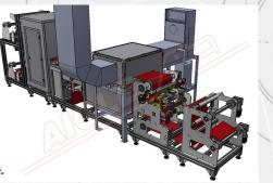
The fabric or substrate is twisted through unwinders and in case also accumulators. The accumulator can hold several linear meters of fabric, providing enough time to replace the empty roll with a new one without stopping the coagulation line.
