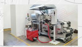
Coagulation lines are used for the production of filters and synthetic leather. This is a wet process. The substrate is first impregnated or squeegeed or slotted and then placed in contact with water diluted with other chemical compounds.
