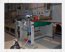
The Rotary Screen Coater mod. BS1/T is used to coat and print fabric (with pigments, resin and adhesives), and for pattern flocking.
