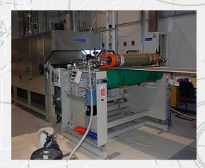
The Rotary Screen Coater mod. B\$1/T is used to coat and print fabric (with pigments, resin and adhesives), and for pattern flocking.
