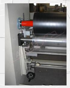
The unit can be used both for air-coating, coating on cylinder, and coating by photoengraved cylinder; it is also equipped with a motorized device to adjust the coating thickness through digital displays.
