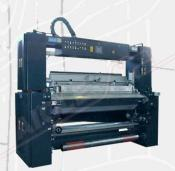
The **Coating Head mod. BS2/M** has been designed and built so that different coating techniques can be employed.
