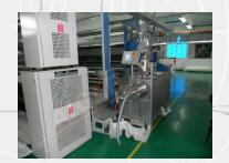
The unit can be used both for air-coating and coating on cylinder, and is equipped with a motorized device to adjust the coating thickness, through digital displays.
