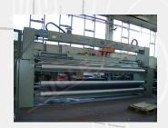
The unit can be used for both air-coating and coating on cylinder and it is equipped with a motorized device to adjust coating thickness through digital displays, and to lift the blade when the seam passes through.
