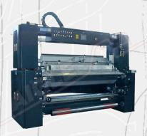
The Coating Machine mod. BSR/M is used to coat fabric (with resin and adhesives).
