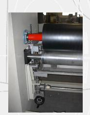
The **Coating Machine mod. BSR/M** is used to coat fabric (with resin and adhesives).
