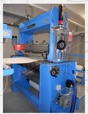
The Coating Machine mod. BSR/R is used to coat fabric, paper and TNT (with resin and adhesives).
