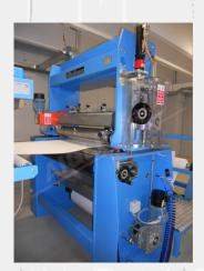
The Coating Machine mod. BSR/R is used to coat fabric, paper and TNT (with resin and adhesives).
