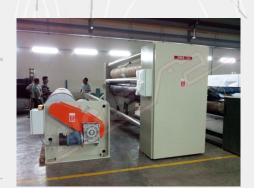
The Calendering Unit mod. GG/IR can operate with hot or cold calendering roll.
