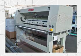
The **Powder Distribution Unit mod. TDP/M** consists of one hopper containing powder, with an inverter-controlled dosing cylinder of adjustable speeds placed at its base.
