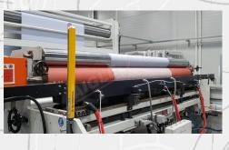
Application systems for **hot-melt laminating** lines: Smooth or engraved cylinder system Slot system.
