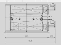
The stenter has an inverter equipped A.C. motor with a local potentiometer for line synchronization with the other elements in the line.
