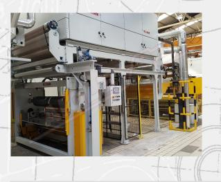
A gap micrometric adjustment system between the printing roller and the back up roller and a stainless steel tray containing the ink and scraper blade comes with adjustable inclination and pressure. At least a couple of pneumatical pistons for the quick lifting and lowering of the whole system (printing roller, motorization and tray); in this way it is possible to keep rotating the printing roll also when it is lowered, in order to prevent the drying of the ink.
