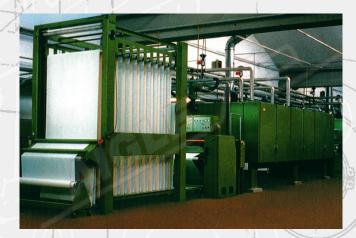
Synthetic leather is obtained by coating on release paper layers of PVC and/or polyurethane (PU).
