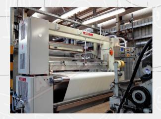
The paper, after detachment from synthetic leather, is rewound carefully and re-used several times in the production process until its replacement is necessary.
