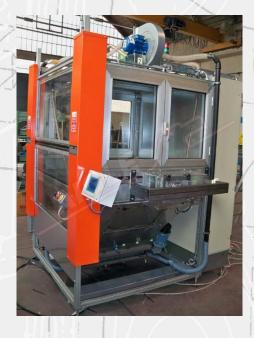
The cabinet is part of a range of machines and lines specifically designed for flocking objects for high productivity. Particular attention was given to the automotive industry, which requires high standards for:
