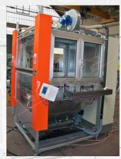
The Automatic 3D Object Flocking Cabinet – mod. CA-ESP can flock a high variety of objects with different shapes.
