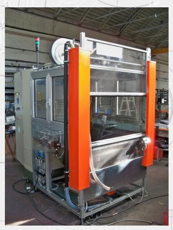
The Automatic 3D Object Flocking Cabinet – mod. CA-ESP can flock a high variety of objects with different shapes.
