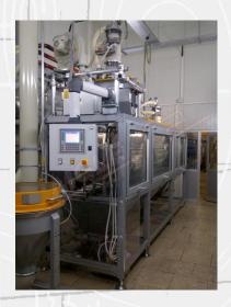
The **Jet-Matic** unit consists of a series of compressed air nozzles, placed above and below the profile. Air flow and pressure, as well as nozzle orientation, are easily adjustable. The unit is connected to the central suction system through hoses. Normally the suction system consists of a suction fan connected to air intakes, to flocking machine suction hoppers, and to a wide-surface filter integrated in the conditioning system.
