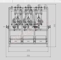
Each brush is equipped with its own electrical motor, compressed air nozzles for profile cleaning and a suction hood for dust recovery.
