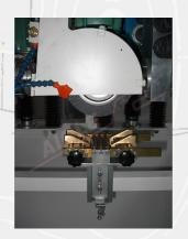
The **Sanding Machines mod. SUC3 and SUC2+1** are specifically manufactured to sand profile surfaces where adhesives will be deposited.
