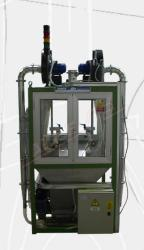
The Electropneumatic Flocking Machine mod. FR/ESP is designed for the flocking of profiles with undercuts.
