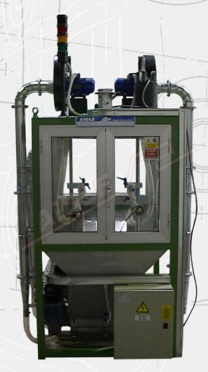
The Electropneumatic Flocking Machine mod. FR/ESP is designed for the flocking of profiles with undercuts.
