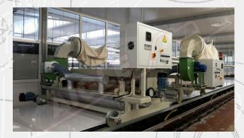
Glitter Distribution Unit The mod. consists of one hopper containing glitter, with an inverter controlled dosing cylinder of adjustable speed placed at its base. A doctor blade opposed to the cylinder is used to adjust the glitter output. A rotating brush is mounted opposite to the cylinder and is used to remove the glitter distribute it onto the underneath. Brush speed is variable and controlled by an inverter. The unit can be inspected through Plexiglas panels.
