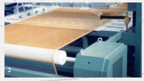
A pre-feeder placed on top of the machine stores the flock and constantly feeds it to the flocking hoppers. Flock levels inside each flocking hopper is controlled automatically.
