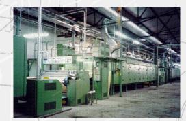
**Drying Oven for Coating Lines mod. FOP/C**'s main features are:
