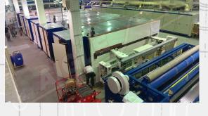
Oven structure, this has silicone rubber sealing doors that are positioned all along the sides in order to grant easy inner access. Both the side doors as well as the upper coverings are made of sheet-zinc panels containing high-density mineral wool. The oven is built in order to guarantee maximum sealing and insulation.
