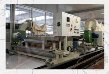
The Glitter Distribution Unit mod. TDP consists of one hopper containing glitter, with an inverter controlled dosing cylinder of adjustable speed placed at its base. A doctor blade opposed to the cylinder is used to adjust the glitter output. A rotating brush is mounted opposite to the cylinder and is used to remove the glitter and distribute it onto the fabric underneath. Brush speed is variable and controlled by an inverter. The unit can be inspected through Plexiglas panels.
