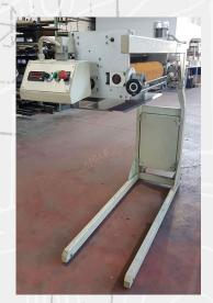
The Glitter Distribution Unit can be used alone or combined with a Flocking Group mod. TC2 (see scheme below).
