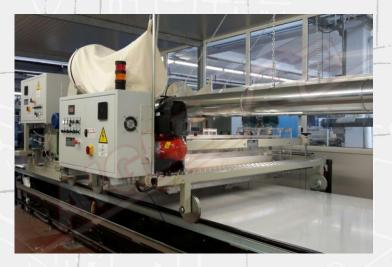
The **Flocking Trolley mod. TCR/COMPL** has to be assembled on the end shoulders of a flat screen printing machine. The flocking trolley runs back and forth on two rails mounted on the printing machine's shoulders. The trolley and printing machine speeds are synchronized. While fabric stops between printing phases, the trolley flocks the fabric which lies underneath.
