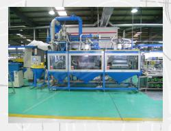
A flock distribution section, consisting of a longitudinal flocking hopper containing a rotating brush. The brush is opposed to a wire mesh frame that can be easily removed for cleaning. Brush rotation speed can be adjusted and a motorized system allows for the adjustment of hopper height, relative to the profile as well.
