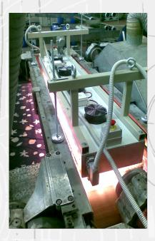
**Infrared Pre-Drying Oven** has been designed for different purposes:
